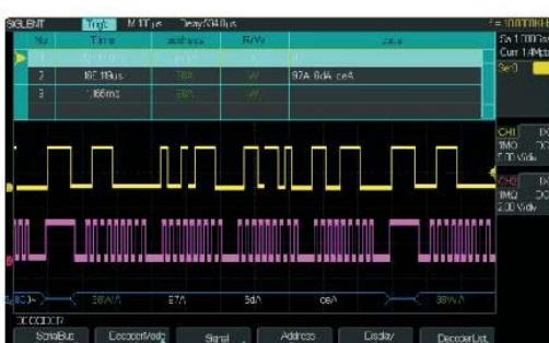
Serial protocol decoding show directly on the waveform with an intuitive, color-coded overlay and presented in binary, hex or ASCII.
